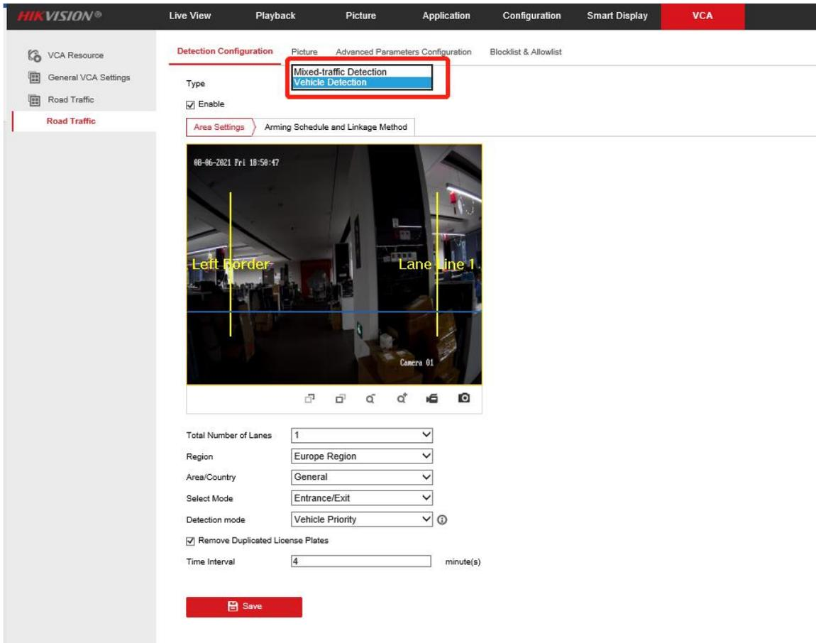
Detection type can be set as Vehicle detection or Mixed-traffic Detection.
