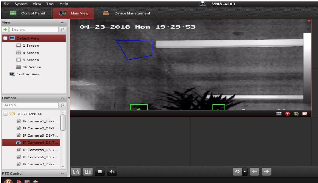
3. Select one channel, and click the right mouse button. Click **start two-way audio**, there will be two options, **Camera1** and **Camera 2**. It means the NVR has two two-way audio channels, **channel1** and **channel2**. You can select one of them to start two-way audio.
