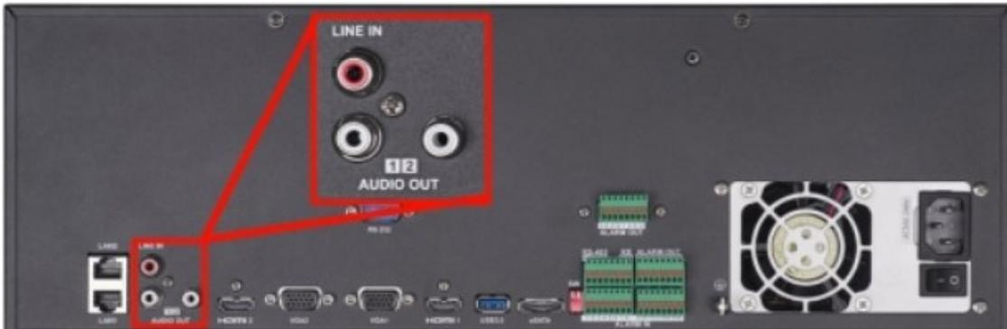
3. HDMI port can transmit audio signal, so HDMI port works as an independent two-way audio port in NVR which support HDMI/VGA asynchronous output. However, VGA port can't transmit audio signal, so it has to be linked with one audio out port. For example, DS-7700NI-I4, this model has one audio output ports and one HDMI port. So in the webpage of NVR, there are two two-way audio channels for choice.
